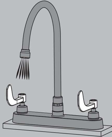
**7** Install the Trim Sleeves (1) over the spindles, followed by the Handles (2), Lock Washers (3), and secure with Handle Screws (4). Install Index Buttons (5) into handles (Blue on right handle, Red on left handle).
