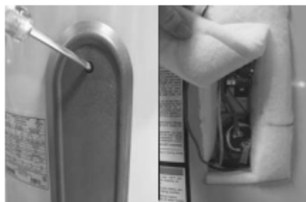
Figure 45 - Element Access Panel/ECO Compartment
