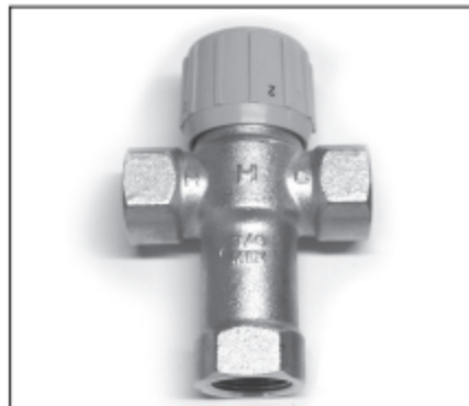
Figure 24 - Adjust Thermostatic Mixing Valves at each point-of-use to 120°F/49°C or lower.
