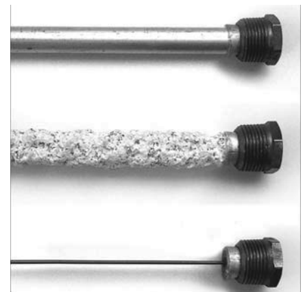
Figure 34 - Anode Rods from new (top) to partially depleted (middle) to fully depleted stages (bottom)
