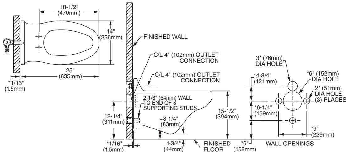
\* THESE DIMENSIONS MUST BE MAINTAINED FOR PROPER INSTALLATION
