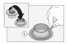
5) Insert flange (L) into drain opening. From below, attach drain body (Q) with gasket (M) and washer (N) to flange (2-3 turns until hand tight).
