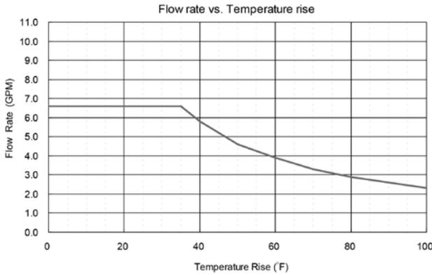
Maximum flow rate is limited to 6.6 GPM.
