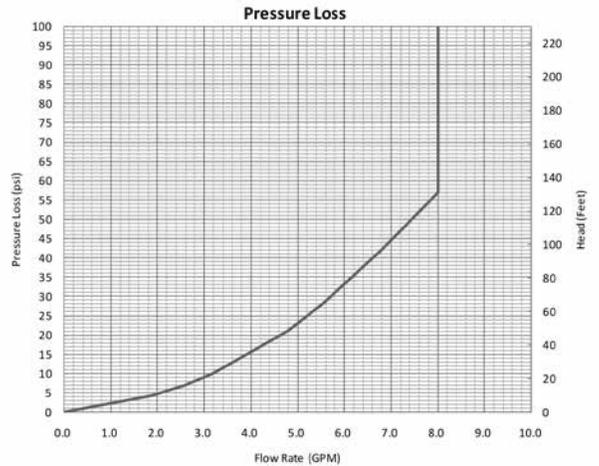
Flow rate is limited to 8.0 GPM.
