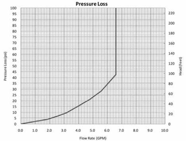
Flow rate is limited to 6.6 GPM.
