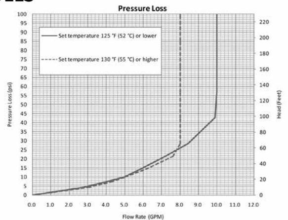
When the set temperature is 125 °F (52 °C) or higher, maximum flow rate is limited to 8.0 GPM.
