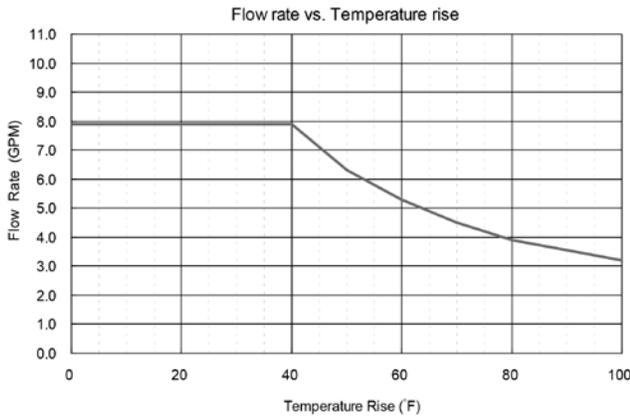
Flow rate is limited to 8.0 GPM.
