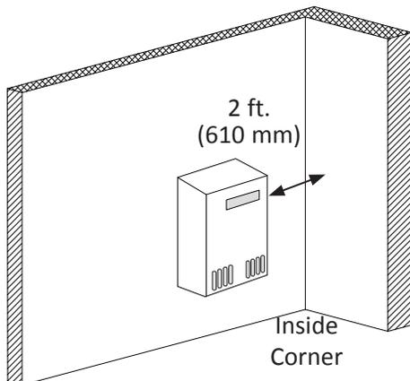
Do not install next to a dryer or any source of airborne debris that can be trapped inside the combustion chamber, unless the system is direct-vented. The air intake must maintain a safe distance from the dryer's exhaust vent. This will help to prevent lint from being drawn into the water heater's air intake.
