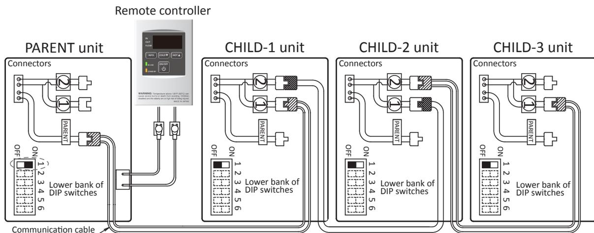
**NOTE:** The dark square indicates the correct DIP switch position.
