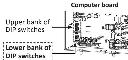
**NOTE:** The tables above show the correct DIP switch position for each temperature setting. (Each black square represents a switch.) For the 110U (AT-KJr3U-IN/OS) and 310U (AT-K5U-IN/OS), only adjust DIP switch No. 9. For the 510U (AT-D3U-IN/OS), only adjust DIP switch No. 5 on the lower bank. Do not adjust the other DIP switches for temperature adjustment.
