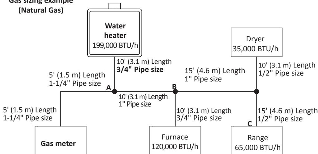
Based on Energy Content of 1,000 BTU/Cubic ft: Divide each appliance's BTU/h requirement by 1,000 BTU/ft<sup>3</sup> to get the appliance's ft<sup>3</sup>/h requirement. Take into account the distance the appliance is from the gas meter, then look in the above gas chart to properly size the line.
