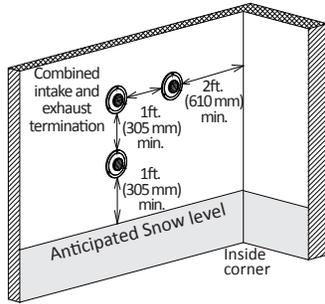
For multiple-unit, direct-vent sidewall terminations that combine the intake and exhaust into a single penetration, space each direct-vent termination at least 1 ft. (305 mm) away from each other, no matter the orientation. A direct-vent termination must also be at least 2 ft. (610 mm) away from an inside corner. If the adjacent wall is less than 2 ft. (610 mm) of length, the minimum required distance away from the inside corner will be equal to the length of that adjacent wall.
