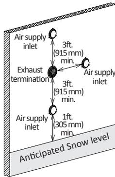
For direct-vent sidewall terminations that use two separate penetrations for the intake and exhaust, distance the intake and exhaust terminations at least 3 ft. (915 mm) away from each other, no matter the orientation unless they follow case 1 and 2 on p. 23.
