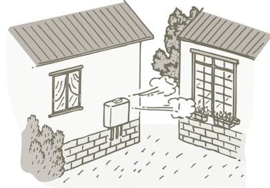
Do not install this water heater under an overhang less than 3 ft. (914 mm) from its top or eaves. The area under an overhang must be open to three sides (Outdoor models only).
