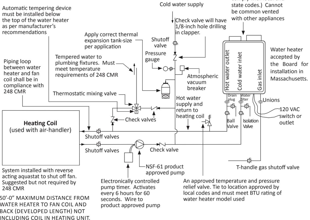
*The recirculation pump is to provide no less than 2 GPM (7.5 L/min) and no more than 4 GPM (15 L/min) through each activated unit in the system*
