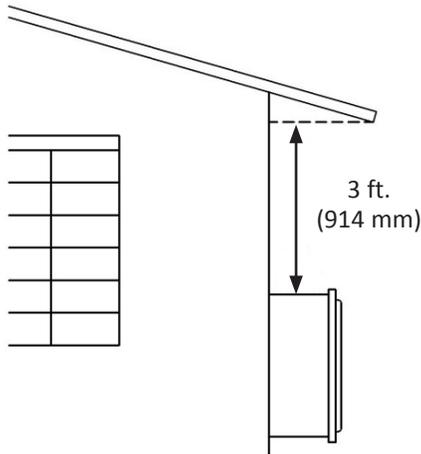
Do not install the water heater direct vent terminator within 1 ft. (30 cm) in the USA of any air intake or building opening, and within 3 ft. (91 cm) in Canada of any air intake or building opening ( Refer to pp. 24 and 25.).
