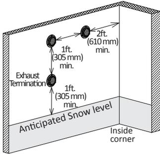
For multiple sidewall exhaust terminations (e.g. multi-unit systems), an exhaust termination must be at least 1 ft. (305mm) away from another exhaust termination. An exhaust termination must also be at least 2 ft. (610 mm) away from an inside corner. If the adjacent wall is less than 2 ft. (610 mm) of length, the minimum required distance away from the inside corner will be equal to the length of that adjacent wall.
