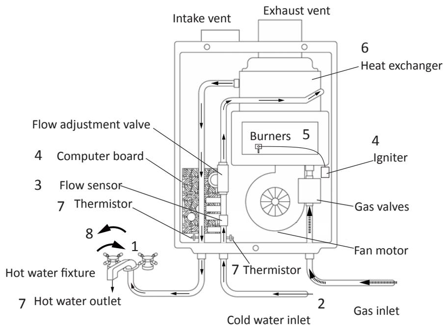
\*This diagram illustrates tankless water heater design concepts only and does not accurately represent the water heater's physical description.
