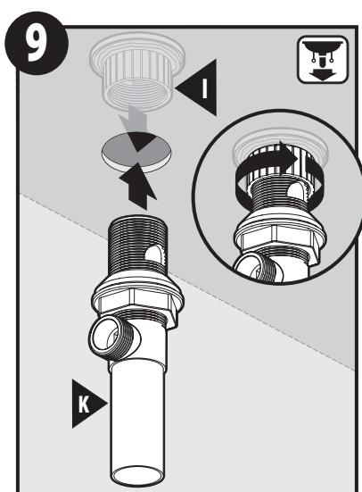
From the underside of the sink, thread the drain body (K) into the waste seat (I).
