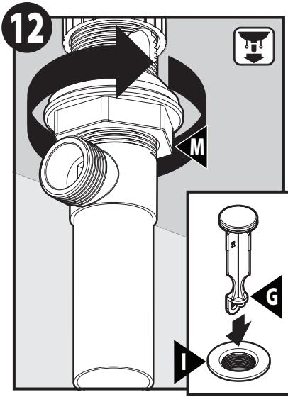
Tighten drain nut (M) and drop plug (G) into waste seat (I) as shown.
