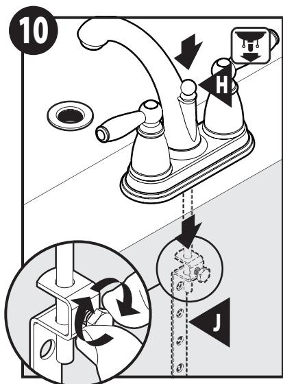
Install lift rod (H) into opening on the top of the faucet. Slide the lift rod strap (J) onto lift rod and tighten the bolt finger tight. Final tightening will be completed during Step 14.
