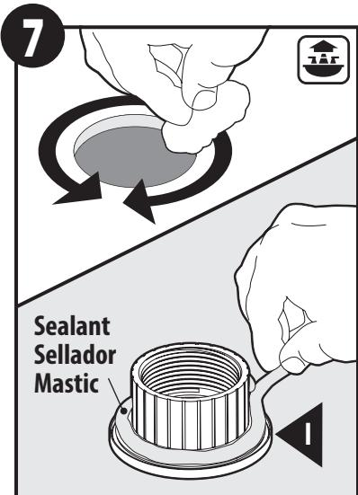
Clean drain opening in the bottom of sink. Apply a generous amount of sealant to the underside of the waste seat (I).
