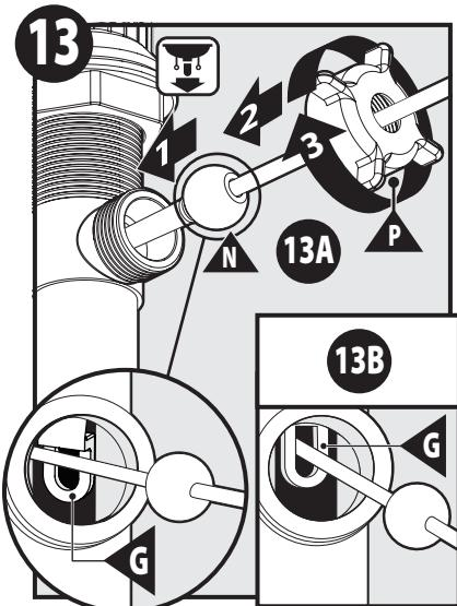
The pivot rod (**N**) can be installed in two ways. Illustration (12A) shows the pivot rod (**N**) next to hole in plug (**G**). This allows the plug (**G**) to be pulled out for cleaning. Illustration (12B) shows the pivot rod (**N**) inserted into the hole in the plug (**G**). This prevents the plug (**G**) from being easily removed after installation. Once the pivot rod is installed (12A or 12B), tighten the pivot rod nut (**P**).
