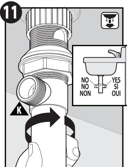
Rotate pivot rod opening on side of drain body (K) to face towards wall as illustrated.
