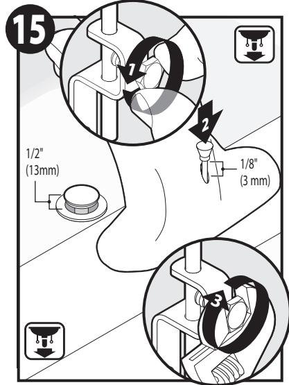
1. Loosen nut on strap (**J**) to allow lift rod to rest in faucet.
