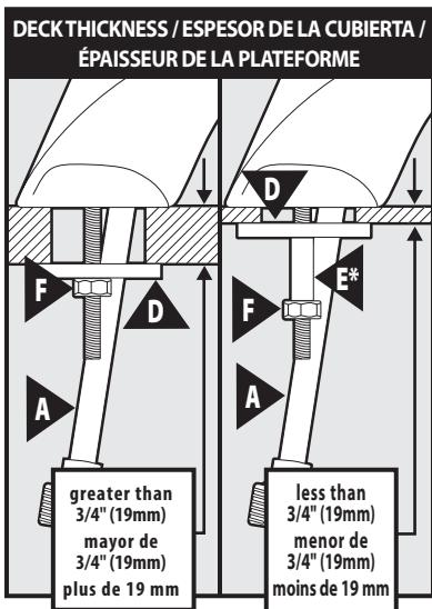
Depending on deck thickness, the Spacer Sleeve (E)\* may or may not be needed for mounting and securing faucet to the sink.
