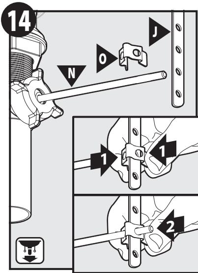
Push pivot rod (**N**) down. Slide one side of clamp (**O**) onto pivot rod. Insert pivot rod through closest hole on strap (**J**) with pivot rod down. Squeeze clamp and slide other side of clamp onto the pivot rod.
