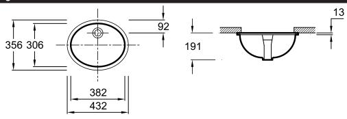
Product Specification: Undercounter basin oval, 43 x 36 cm. 2209. Collection: CAXTON. Dimensions: 43 x 36. Weight: 7.7 kg. Material: Ceramic. Installation: Undercounter. Faucet drilling: No faucet hole. Install this Caxton undercounter lavatory beneath solid-surface countertops to combine the look of an integral basin with the benefits of durable vitreous china. Caxton lavatories complement both traditional and contemporary décor.
