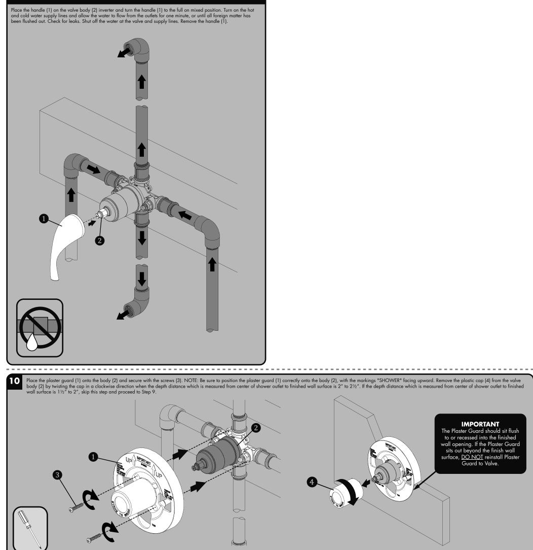
IMPORTANT The Plaster Guard should sit flush to or recessed into the finished wall opening. If the Plaster Guard sits out beyond the finish wall surface, <u>DO NOT</u> reinstall Plaster Guard to Valve.
