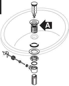
Mount the drain assembly (not included) on the sink, following faucet manufacturer's instructions. Be certain to apply a bead of sealing putty on the underside of the drain (Part "A") in order to ensure a watertight seal between the sink and drain. Remove excess putty after installing drain on sink.
