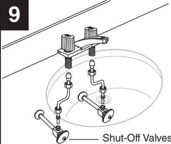
Connect supply line to faucet (finger tight) and carefully bend tubes to engage with the supply shut-off valves. Tighten connections at faucet and shut-off valves for water tight seal.
