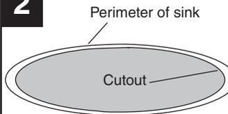
Carefully cut out the enclosed template, then position and trace the template on the countertop as shown on the template. Make a mark of the faucet hole centerline on the countertop. Drill a 1/2" pilot hole on the inside of the cut line. Use a saber saw or a keyhole saw to cut out the countertop opening.
