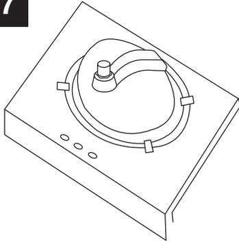
Center bowl over cutout and tighten screws (see step 4) to secure bowl to countertop. Remove excess sealant from inside lip.
