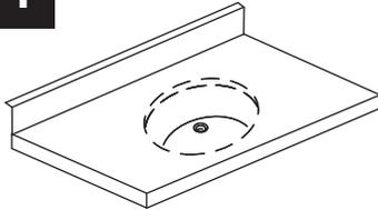
**NOTE:** To avoid damage to countertop, install sink such that future removal from underneath the countertop is possible.
