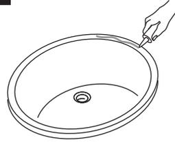
After checking fit and alignment of sink to cut out, apply a bead of silicone caulking/adhesive to rim of sink.
