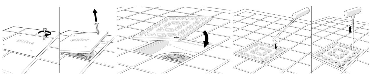
IMPORTANT! Allow new grout to cure 24 hours before removing construction plug
