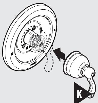
After setting the adjustable temperature limit stop to the desired position, reattach the Handle (K).
