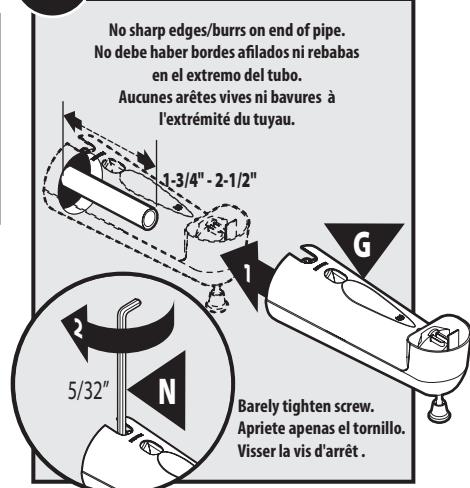
1. Install Tub Spout (G) upside down onto pipe.
