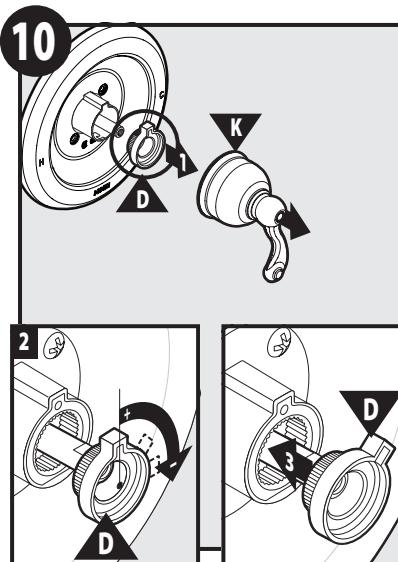
Remove the Handle (K). Note the position on the stop. Position the Adjustable Temperature Limit Stop (D) so the Lever stops at the position. This prevents the Lever from being turned into an unsafe temperature.
