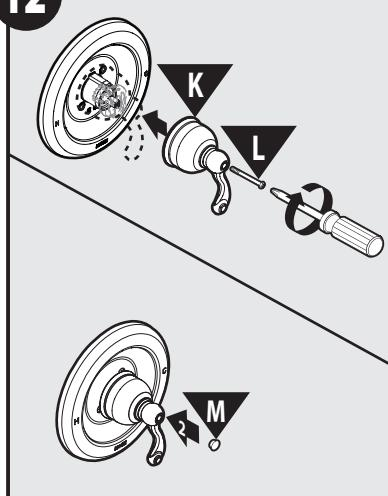
Insert Screw (L). Tighten screw and insert Handle Cap (M).
