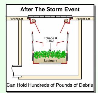
The coarse screen provides additional filtered flow with less chance for obstruction than either the medium or fine screen. The coarse screen is sized to capture floatables like foliage and litter. At this stage water is flowing through all the different sieve size screens, the *turbulence deflector* continues to dramatically reduce the turbulence in the lower filtration chamber, and sediment continues to settle and collect toward the bottom.
