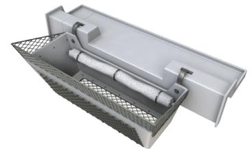
Standard Capacity Curb Inlet Basket with built in shelf system allows for ease of installation and service. Typically used in shallow catch basins.
