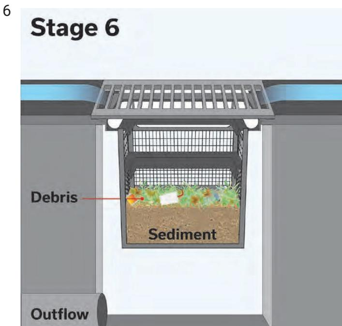
After the storm event has subsided, the stormwater will drain from the GISB completely leaving all collected debris suspended in the screen system to dry until removal during service. The screen also contains the nutrient pollutant load while also prevent septic water, mosquito breeding and nutrient leaching.
