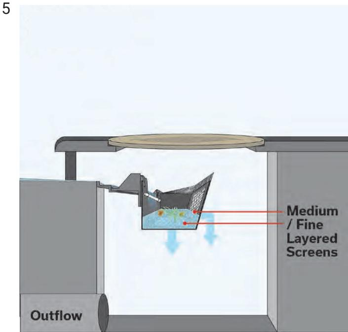
After the storm event has subsided, runoff will drain from the CIB leaving all collected debris suspended in the screen system to dry until removal during service. Captured pollutants include trash, debris, sediment as well as the nutrient pollutant load which prevents septic water, mosquito breeding and nutrient leaching.
