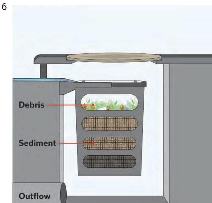
After the storm event has subsided, the stormwater will drain from the HCCIB completely leaving all collected debris suspended in the screen system to dry until they are removed at time of service. The dry state storage contains solid debris as well as the nutrient pollutant load while also working to prevent septic water, nutrient leaching and mosquito breeding.
