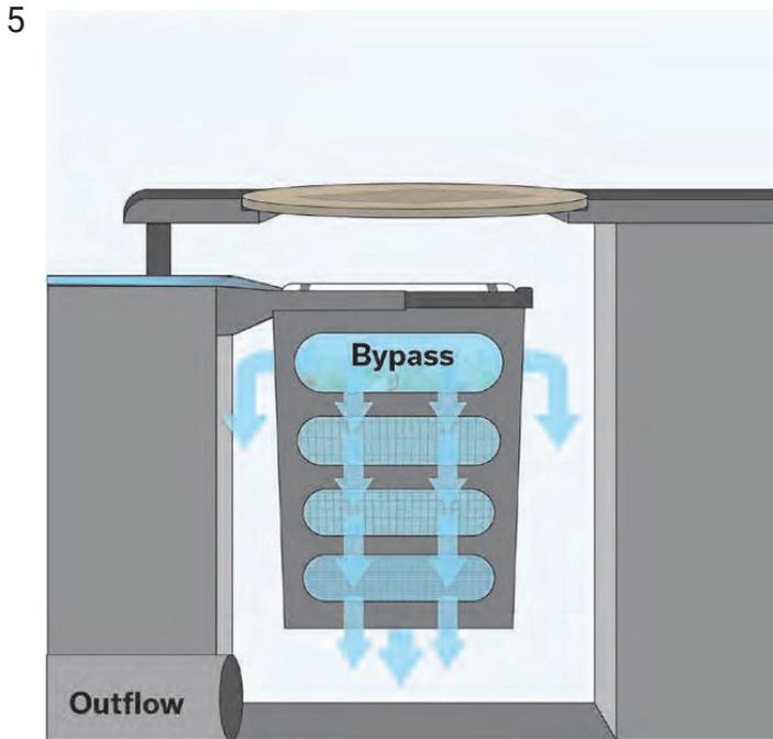
If the stormwater flow rate is extreme or the unit is full where the flow rate exceeds flow through all the screens, the water will bypass the screens through skimmer protected openings at the top of the HCCIB. During this time, water flow is still partially treated and continues to pass through all filtration screens.
