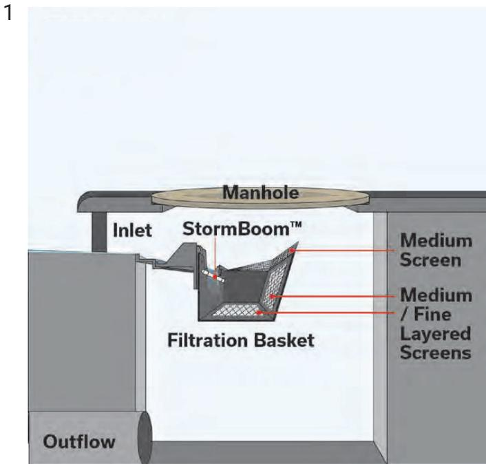
Stormwater enters the inlet immediately coming in contact with a StormBoom which absorbs floating oils and hydrocarbons. The StormBoom can be outfitted with multiple types of filter media and is installed just under the weir opening.
