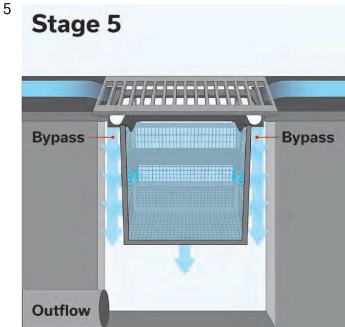
If the stormwater flow rate is extreme or the unit is full where the flow rate exceeds flow through all the screens, the water will bypass the screens through skimmer protected openings at the top of the GISB.
