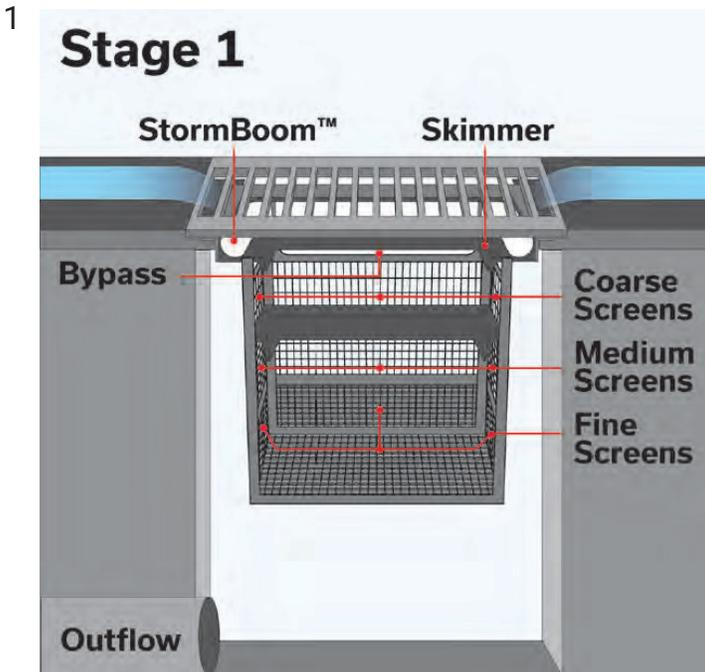
Stormwater enters the grate inlet immediately coming in contact with a StormBoom which absorbs floating oils and hydrocarbons. The StormBoom can be outfitted with four types of filtration media and is installed at the top of the device.
