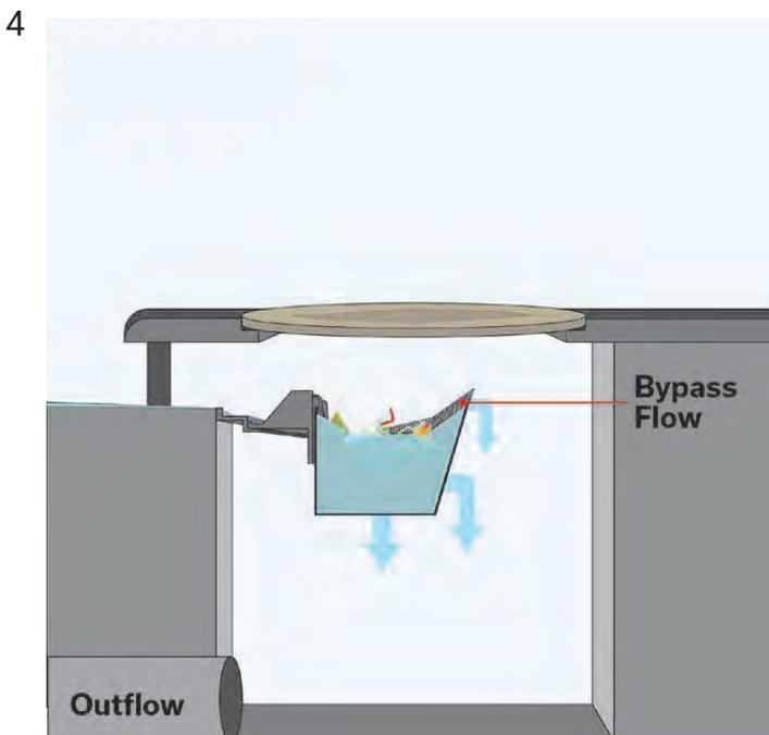
As stormwater continues to flow into the filtration basket, sediment and debris continue to accumulate. As storm flow intensifies and / or the basket fills, water will begin to filter through the side screen in addition to the lower screens.
