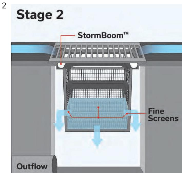
Throughout the storm event, water continues to come in contact with the StormBoom and then flows into the lower filtration chamber adjacent to the fine sieve size screens. The fine sieve size screens filter out fine particulates such as phosphates and sand.
