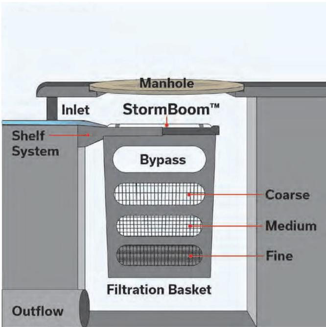
Stormwater enters the curb inlet immediately coming in contact with a StormBoom which absorbs floating oils and hydrocarbons. The StormBoom can be outfitted with four types of filtration media and is installed at the top of the screen basket.
