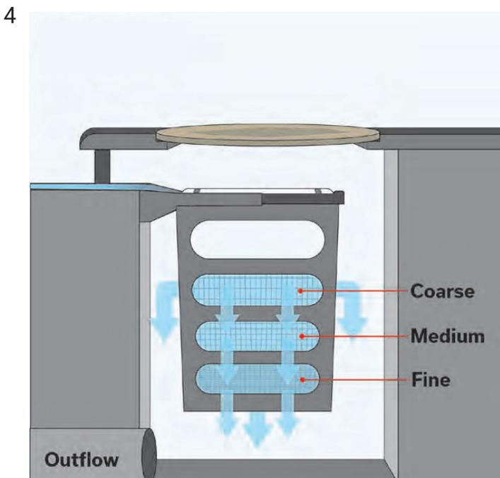
If the storm intensity becomes a high flow event, the water level in the HCCIB rises to a level adjacent to the coarse sieve size screens. These screens provide additional filtered flow with a far less chance of obstruction than the fine or medium sieve screens and is designed to capture floating debris like foliage and trash.
