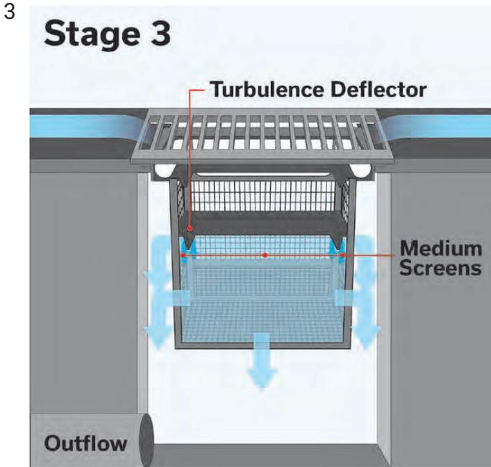
As the storm intensity increases, the water level in the GISB rises to a level adjacent with the medium size sieve screens and turbulence deflector. The medium size sieve screens provide additional flow with less chance of clogs or obstructions forming. The turbulence deflector reduces the turbidity in the lower chamber and prevents scouring.
