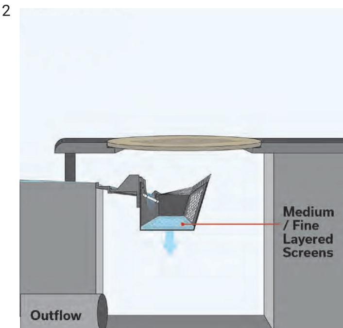
Throughout the storm event, water continues to come in contact with the StormBoom and then flows into the filtration basket where trash, sediment and debris collect. These pollutants are left behind in the basket as the filtered water passes through the bottom screen.
