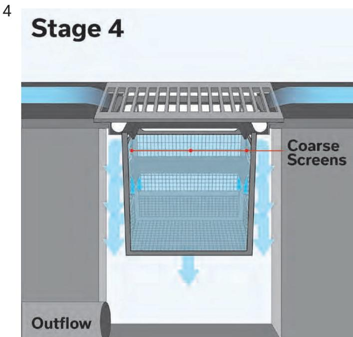
If the storm intensity becomes a high flow event, the water level in the GISB rises to a level adjacent to the coarse sieve screens above the first turbulence deflector. The coarse screen provides additional filtered flow with a far less chance of obstruction than the fine or medium sieve size screens and is designed to capture floating debris like foliage and trash.
