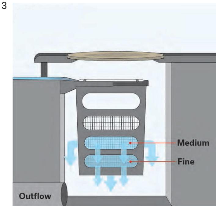
As the storm intensity increases, the water level in the HCCIB rises to a level adjacent with the medium sieve size screens. The medium sieve size screens provide additional flow with less chance of clogs or obstructions forming.
