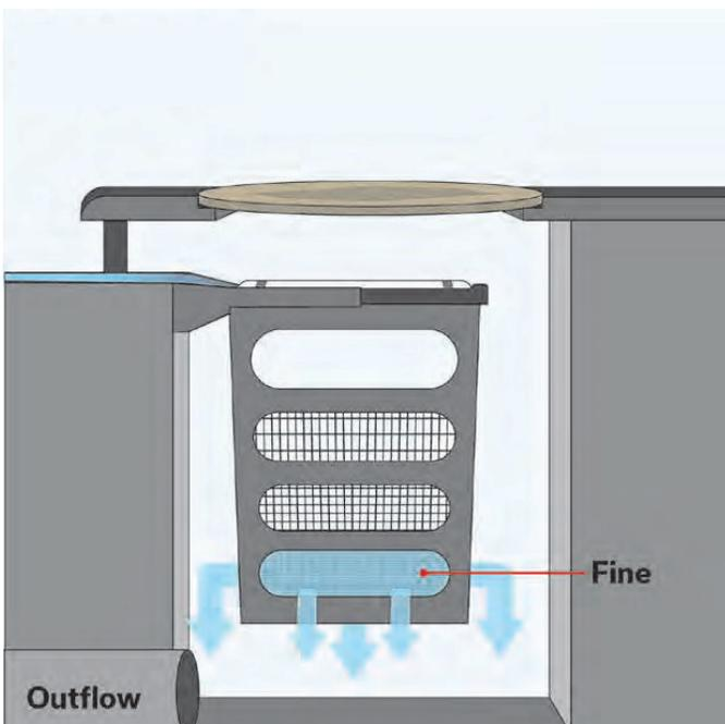
Throughout the storm event, water continues to come in contact with the StormBoom and then flows into the filtration basket where fine particulates and debris begin to settle. These pollutants are left behind in the basket as the filtered water passes through the bottom and lower fine sieve screens.
