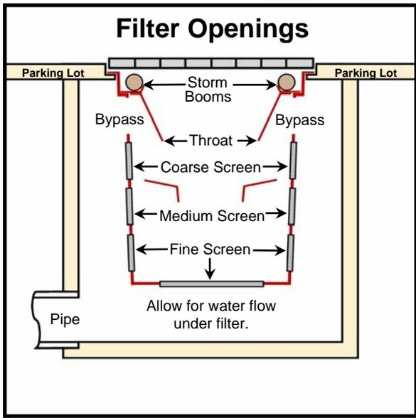
The **maximum flow rate** of a *Grate Inlet Skimmer Box* is determined by the amount of flow that can pass through the throat, the exception is found only in very large units.
