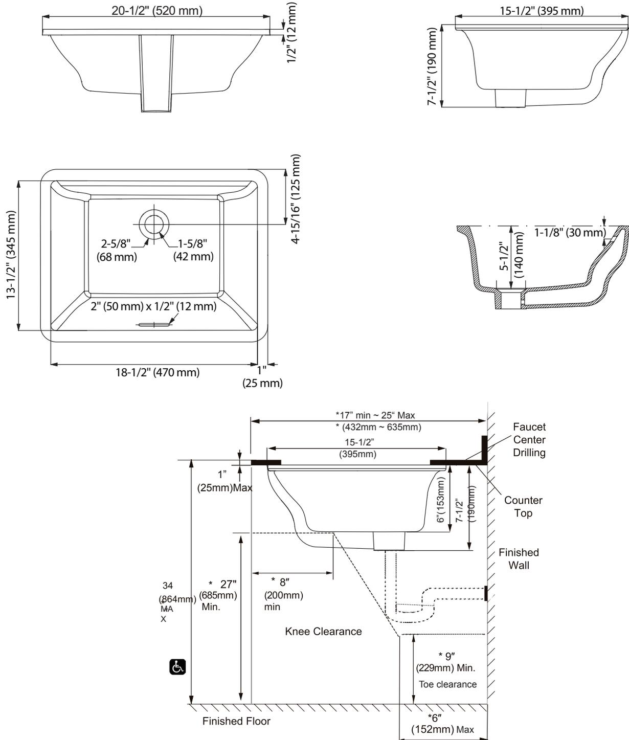
Note: All dimensions and specifications are nominal and may vary: Dimensions of 8" and greater have a tolerances of +3%. Dimensions less than 8" have a tolerances of +5%.
