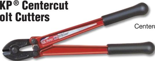
Contractor-quality centercut boltcutter for cutting concrete reinforcing rods, soft and medium hard bolts, rods forged jaws. One-half the weight of traditional boltcutters. One-piece handles attach directly to the jaws. (50) pounds of hand pressure at handle turns into 4,000 pounds of pressure at jaw.
