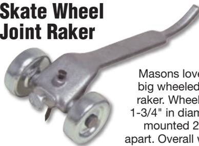
Masons love this big wheeled joint raker. Wheels are 1-3/4" in diameter, mounted 2-1/4" apart. Overall width is 3-5/8". Has 8-1/2" aluminum handle that is squared off at the end so you can rod joints. Hardened nail is adjusted for depth.
