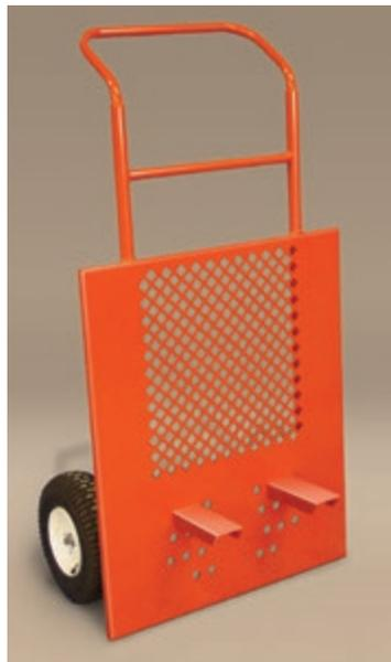
Heavy-duty all terrain cart allows user to move straps of bricks. Comes with 7-1/2" prongs and a heavy-duty 3 piece hub with 2 ply tube type tires. Rubber sealed heavy-duty ball bearings. All steel wheels with grease fittings. Constructed for a lifetime of service. 800 lb. capacity. Must ship by truck (only). Weight: 112 lbs.
