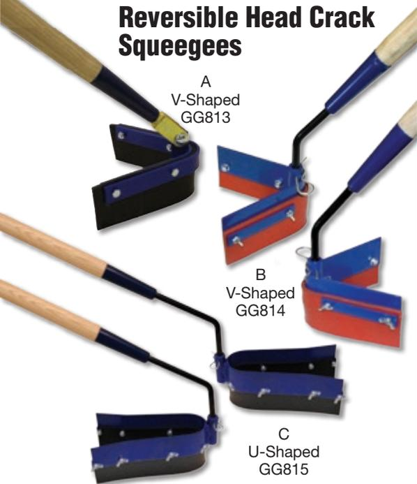
Reversible head allows a push or pull action to funnel material into cracks. Choose between V or U-shaped black Neoprene blade that withstands temperatures up to 220°F. V-shaped red silicone blade withstands temperatures up to 450°F. Each includes a 54" heavy-duty wood handle. Blades are reversible.
