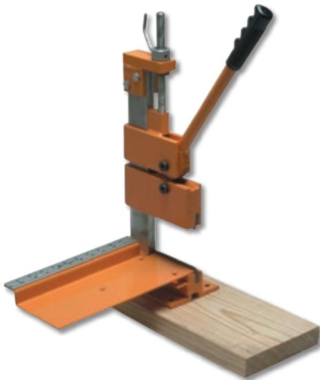
At only 39 lbs this brick splitter easily travels from jobsite to jobsite. The opening is a full 5" high fitting a standard brick standing up at an angle. The lever action increases your arm strength, making cuts with minimum effort. The blades are 4-1/2" wide, so it cuts most bricks now in use. A 12" rule and square is built right into the Mini Splitter for accurate cuts.
