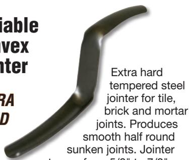
Extra hard tempered steel jointer for tile, brick and mortar joints. Produces smooth half round sunken joints. Jointer tapers from 5/8" to 7/8" on curvature. Legs measure 3-1/2" and 4-1/4" long. Easy to handle tool adjusts to various joint widths.
