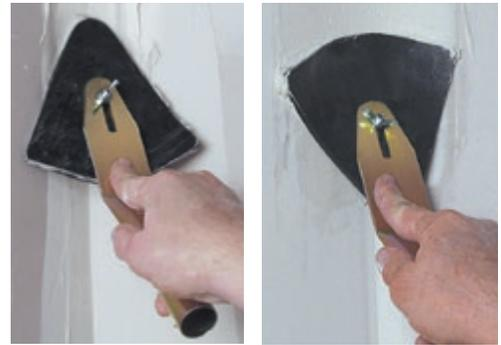
Just loosen nut and rotate for less than 90 degrees or...over 90 degree angles
