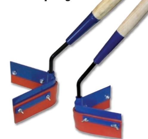
V-shaped head is welded into a fixed position for your choice of either pull or push action. V-shape funnels hot or cold crack filler. Red silicone blade withstands temperatures up to 450°F. Attached to a 54" heavy-duty wood handle (GG814-03).
