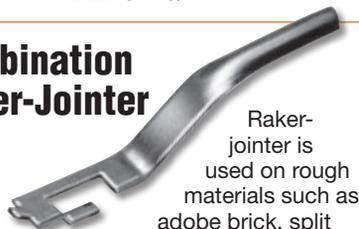
Raker-jointer is used on rough materials such as adobe brick, split stone and split block. It has a 3/4" convex jointer on one end, and a 5/16" raker blade at the other end. Overall length 10".
