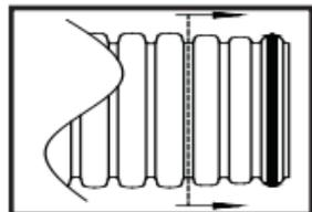
Gasket printing should be visible in this location when properly installed.
