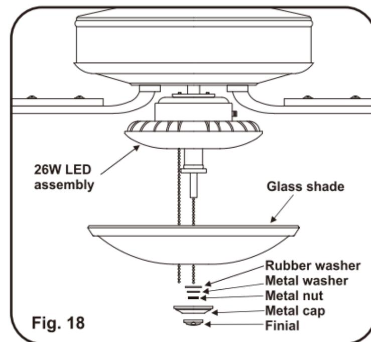
Remarked: the fan is provided extra cap and finial, which can be used when the fan is installed with universal remote control(Not Provided)
