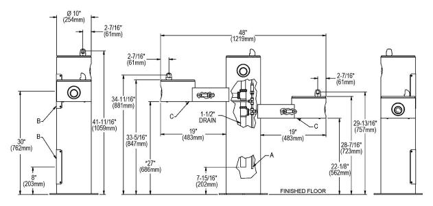
A = 3/8" O.D. Unplated copper tube connect
