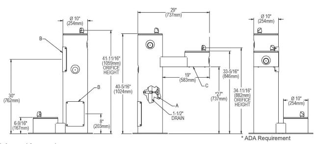
A = 3/8" O.D. Unplated copper tube connect shut off valve by others
