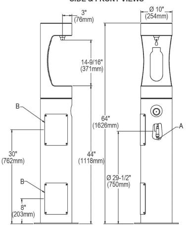
A = 3/8" O.D. Unplated copper tube connect. Shut off valve by others.
