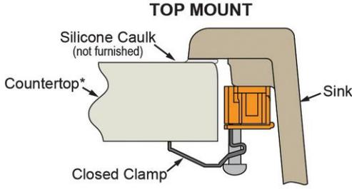
\*Maximum thickness for use of hold down system is 1-3/4" (44mm).
