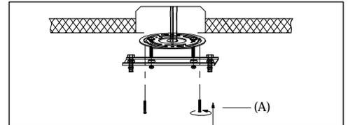
Step.1: Remove mounting bracket (A) from fixture and install to electrical box.
