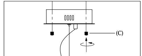
Adjust wire length to desired mounting height and tighten strain relief screws to secure. Install fixture to bracket and tighten screws (C) on the canopy to secure.
