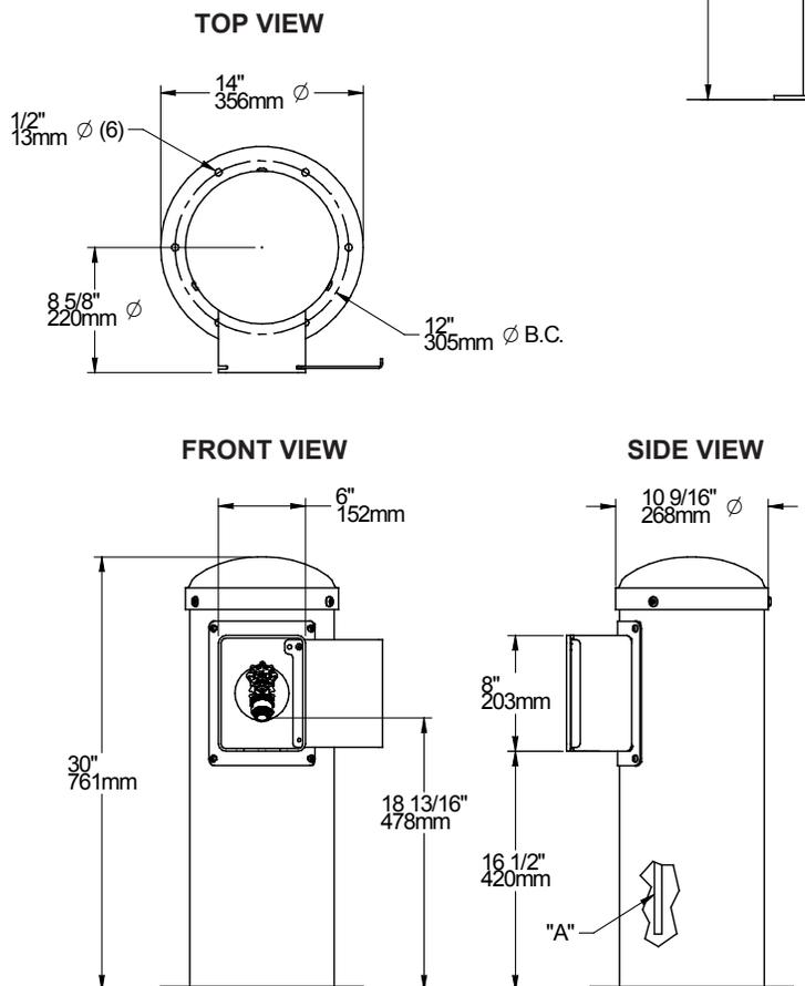
A = 1/2" O.D. UNPLATED COPPER TUBE CONNECT SHUT OFF VALVE BY OTHERS
