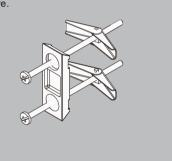
Option A - Tile Wall Insert screws through Mounting Plate and secure Mounting Plate to wall by tightening
