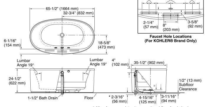
\* Allow for appropriate clearance in subfloor for drain clearance. Note: Horizontal PVC pipe and tee shown, not included.
