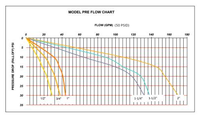
Pressure Differential is the difference between the inlet supply pressure and the adjusted outlet pressure.
