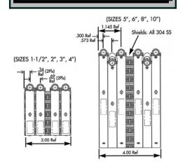
DESCRIPTION: Couplings consist of gasket and shield assemblies. the shield assemblies have four or six clamps depending on size. the clamps are fastened with eyelets to the bi-directional corrugated shield.
