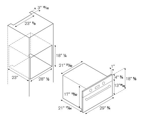
The minimum gap between the kichen cabinet upper or lower panel and the appliance is 1/8. This dimension must be added to the height listed in the drawings
