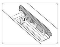
Open the adapter cover to reveal the protective cap of the adapter. Gently pull the cap to the right and lift up to remove.
