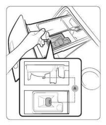
Add fabric softener to the softener compartment. Do not exceed the max line (A).
