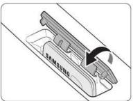
3. Insert the Smart Home Adapter into the Adapter port (A) in the correct direction. Make sure the Samsung logo faces forward.
