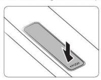
To unlock the adapter cover, press the cover to the left of the word PUSH as shown in the illustration.
