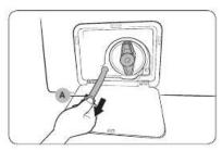
Put an empty, spacious container around the cover, and stretch the emergency drain tube to the container while holding the tube cap (A).
