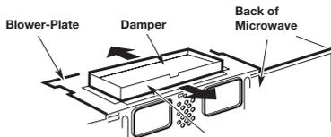
For Front-to-Back Adjustment, Slide the Exhaust Adaptor as Needed
