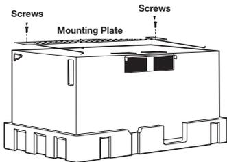
5. Remove the 2 screws from the mounting plate. This plate will be used as the rear wall template and for mounting.
