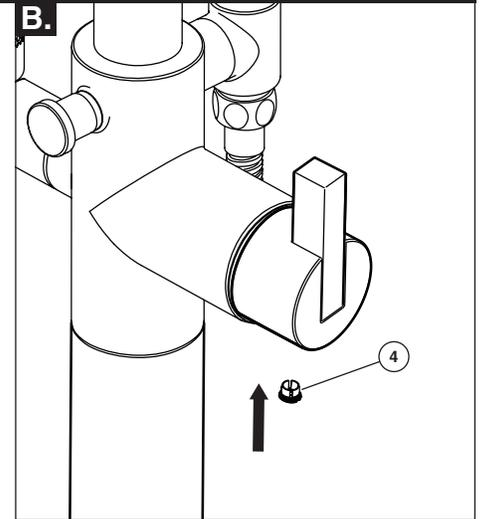
**B.** Position the button cover (4) as shown and push firmly until button is securely flush with handle.
