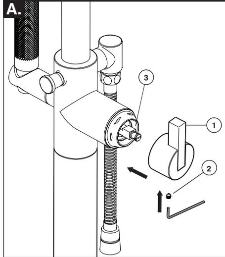
**A.** Place handle (1) over valve stem adapter (3), being careful to align handle. Handle is attached with the supplied set screw (2). Tighten securely.
