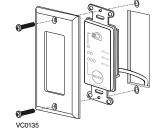
Perform the electrical connection to the terminal connector (**A** or **B**) of the unit, as shown below. For more details, refer to the installation manual of the ventilation unit.
