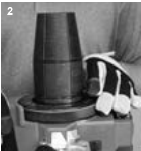
Figure 14: Expander head collar should sit tight against the tool.
