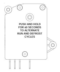
Some refrigerators do not use plug-in connectors for a defrost timer hook-up. Each terminal is connected using a seperate wire. In this case, very carefully bend terminals 2, 4, 3 as illustrated. Use needle-nose plier to hold the terminal while bending it with another plier.
