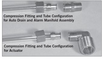
Compression fittings and tubes are provided for connection from the outlet of the auto drain, alarm manifold assembly, and actuator to the drip cup or drain. Install the compression fittings in accordance with the trim drawing provided. NEVER INSERT A PLUG INTO THE OUTLET OF THE AUTO DRAIN, ALARM MANIFOLD ASSEMBLY, OR ACTUATOR IN PLACE OF THE COMPRESSION FITTING/TUBE.
