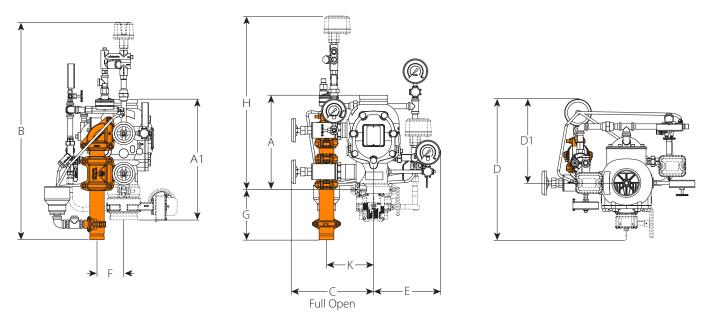
A 4-INCH/114.3-MM VALVE WITH SINGLE-INTERLOCKED PNEUMATIC RELEASE PREACTION TRIM IS SHOWN BELOW 1½ – 2-INCH/48.3 – 60.3-MM CONFIGURATIONS CONTAIN ¾-INCH/19-MM DRAIN VALVES 2½ – 3-INCH/73.0 – 88.9-MM CONFIGURATIONS CONTAIN 1¼-INCH/31-MM DRAIN VALVES 4 – 8-INCH/114.3 – 219.1-MM CONFIGURATIONS CONTAIN 2-INCH/50-MM DRAIN VALVES
