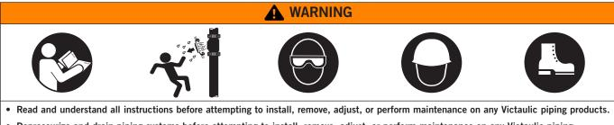
Depressurize and drain piping systems before attempting to install, remove, adjust, or perform maintenance on any Victaulic piping products.
