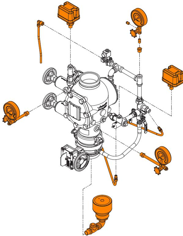
**Electric Release with Series 753-E Solenoid Valve
