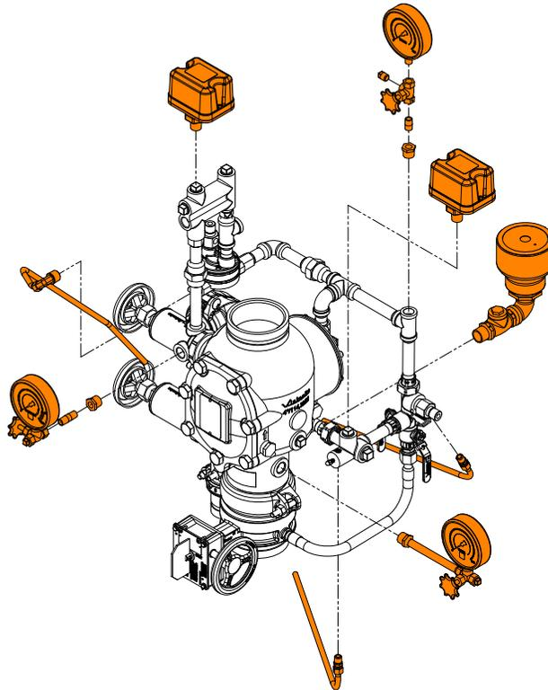
The components shaded in orange below are shipped separate from the valve and must be installed in accordance with the trim drawing provided.
