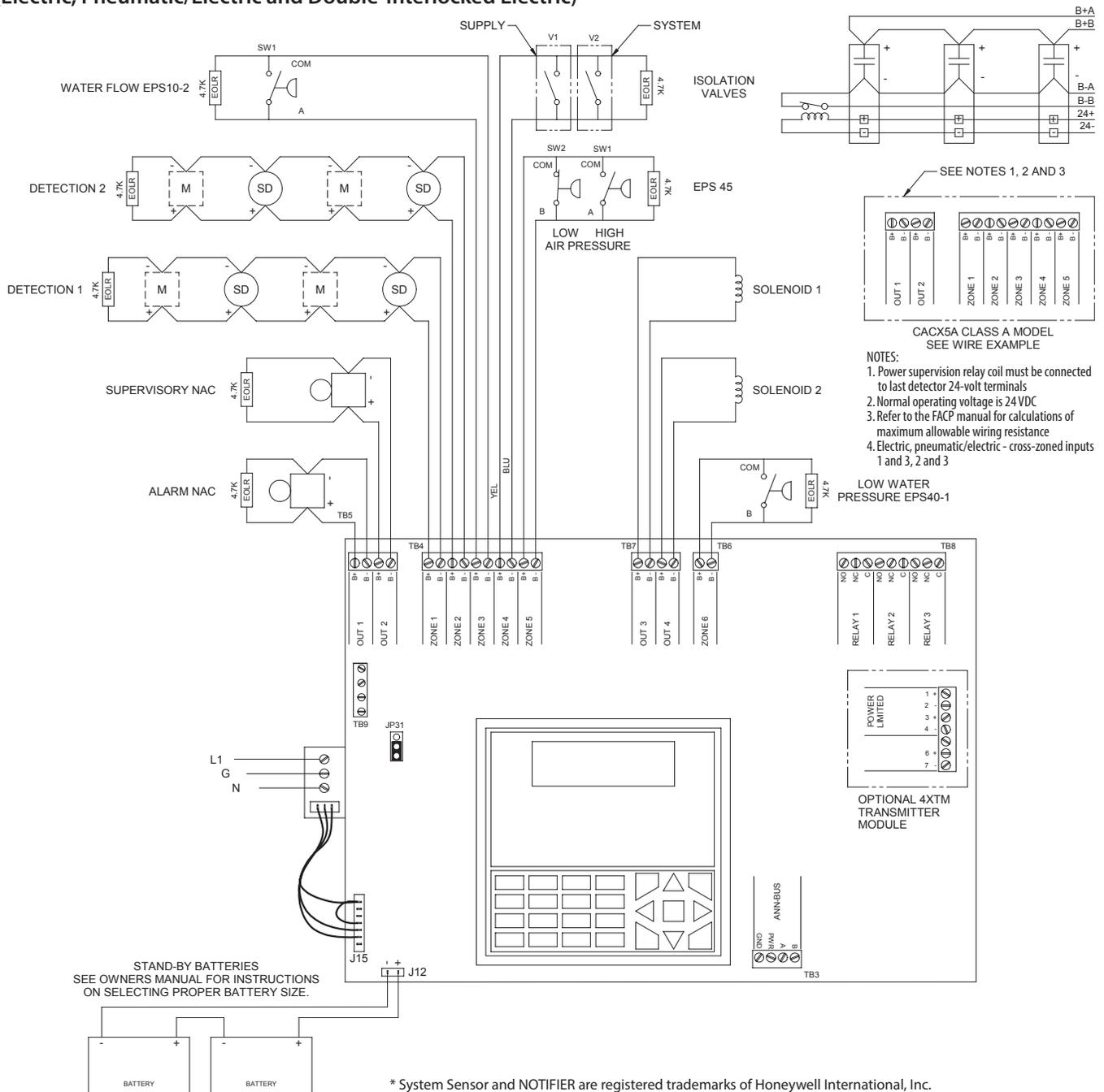
**System Sensor\* PDRP-2001 or NOTIFIER\* RP-2001 Field Wiring Diagram
