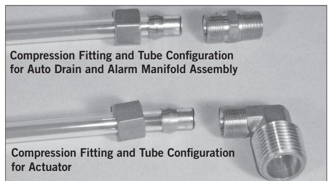
5. Compression fittings and tubes are provided for connection from the outlet of the auto drain, alarm manifold assembly, and actuator to the drip cup or drain. Install the compression fittings in accordance with the trim drawing provided. **NEVER INSERT A PLUG INTO THE OUTLET OF THE AUTO DRAIN, ALARM MANIFOLD ASSEMBLY, OR ACTUATOR IN PLACE OF THE COMPRESSION FITTING/TUBE.**
