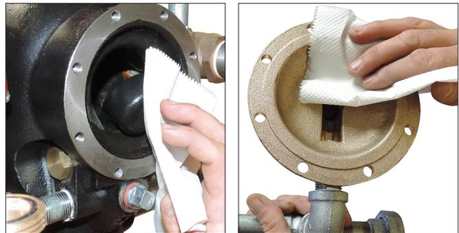
5. Clean the back of the valve body to remove any debris that may interfere with proper diaphragm seating.
