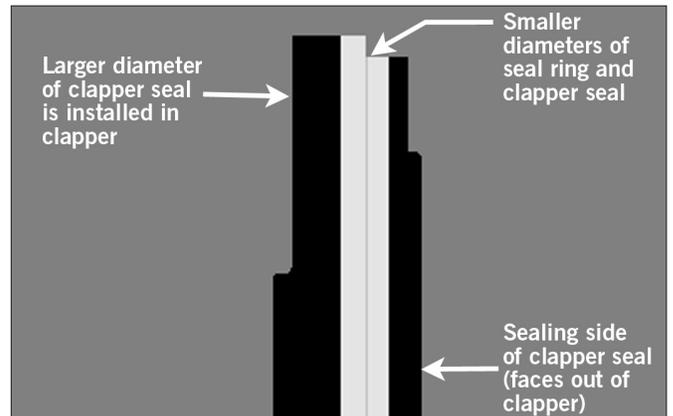
6a. If using the same clapper seal assembly and the seal ring was removed from the clapper seal in the previous step: Re-insert the seal ring carefully underneath the outer lip of the clapper seal. Ensure that the smaller diameter of the seal ring is toward the sealing surface of the clapper seal.
