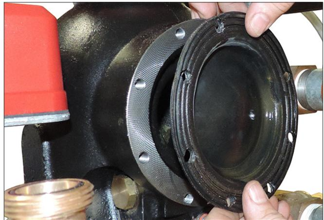
4. Remove the diaphragm from the valve body. Discard the diaphragm.
