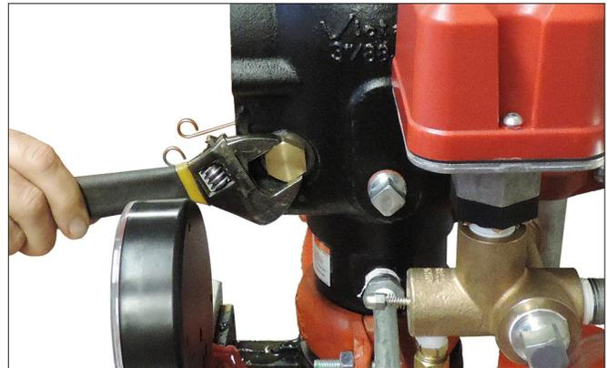
2. Remove the clapper shaft bushings with o-rings from the valve body.
