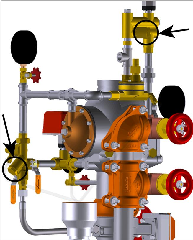
2. Remove the existing cartridge from the air manifold and priming manifold assemblies, shown above. Rinse the cartridges to remove any deposits.
