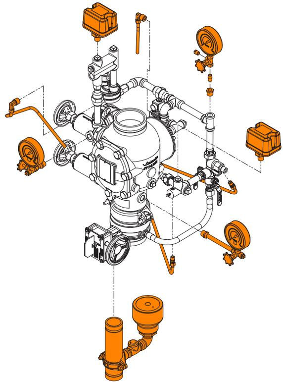
**Single-Interlocked Pneumatic Release with Series 776 Low-Pressure Actuator**
