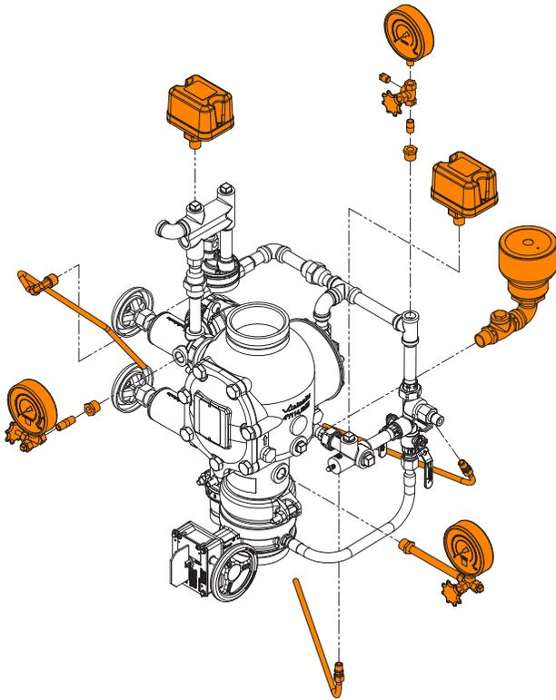
**Non-Interlocked Pneumatic/Electric Release with Series 776 Low-Pressure Actuator and Series 753-E Solenoid Valve**
