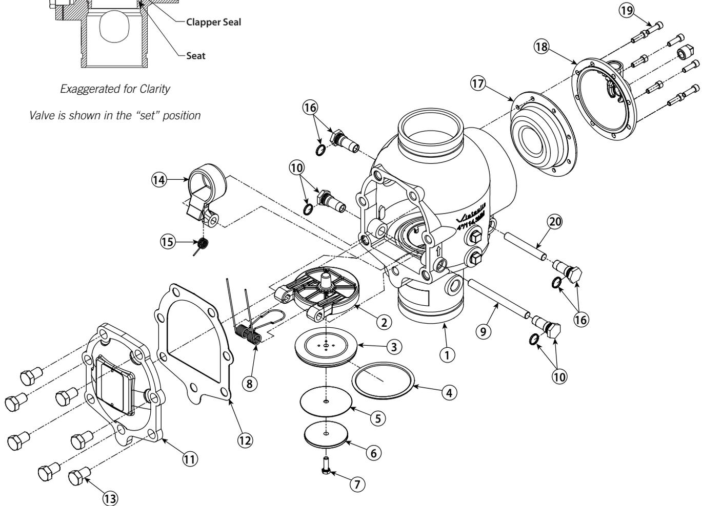
The 1½-inch/48.3-mm and 2-inch/60.3-mm valve sizes contain washers under the heads of the cover plate bolts.
