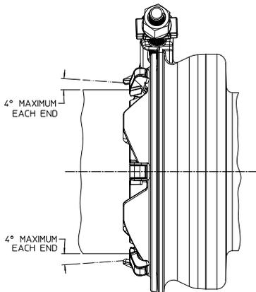
7. Tighten nut until the gasket contacts the pipe and the pipe is snugly held in place. This should happen after applying approximately 10-15 ft-lbs of torque.
