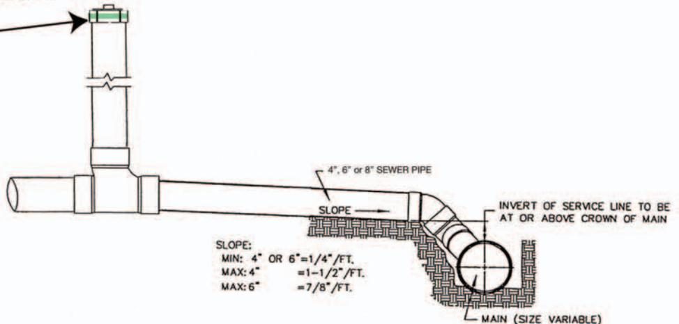
**SPECIFICATION:** Cleanout shall incorporate an electronic disc marker in threaded plug. Disc marker shall be positively retained in plug to eliminate the possibility of separation between disc and plug. Raised plug shall meet all requirements of ASTM-D-3034 SDR 35. Electronic disc marker shall be 3M EMS #1414XR, green in color, with a frequency of 121.6 kHz. Raised cleanout plug with electronic disc marker shall be GPK Products model #228-0004DM, 228-0006DM, 2228-0008DM or approved equal.
