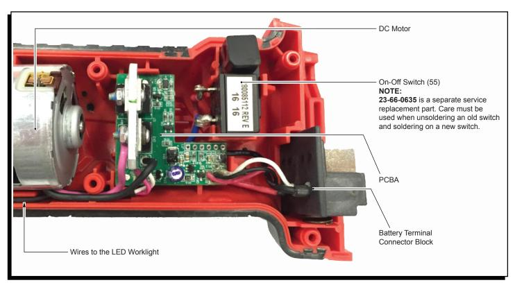
**NOTE:** Be sure to place all components of the Motor/Electronics/Spindle Assembly (52) firmly and squarely in the Housing Support (27). Be sure to route wires into wire traps as shown. Check for any interferences prior to installing the Housing Cover (28).
