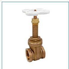
**Specifications UPC** Code 039923355171 Type Gate Valve **Valve Size** 2 in Material Lead Free Silicon Bronze **Description** T111-LF 2 THD 300 CWP RS GATE BRZ Multi-Turn **Turns / Operation** Seat / Seal Material **Bronze Connection Type** T -- Female NPT Thread (FIPT) **Operation Type** Standard Handwheel Weight 5.560 lb
