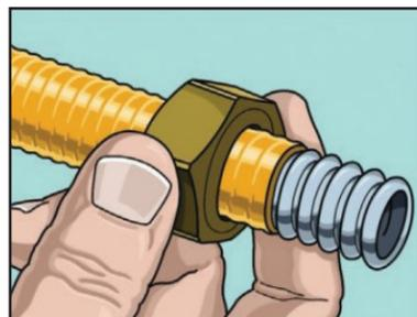
1. Strip and remove plastic coating in the fourth valley and slide on nut.
