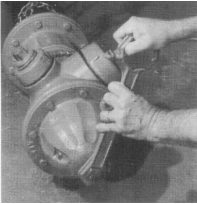
1. Tighten Operating Nut to be sure Main Valve is in the fully closed position.
