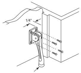
Position stop on door to allow for firm contact with floor and mark position of holes. If pre-drilling is required, use a 3/32 inch drill bit and install as required.
