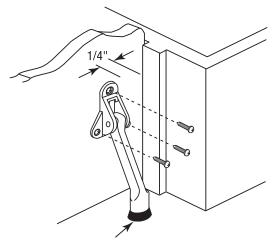
Position stop on door to allow for firm contact with floor and mark position of holes. If pre-drilling is required, use a 3/32 inch drill bit and install as required.
