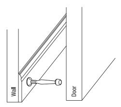
Open your door until it is parallel with the wall. Using a pencil, mark the point on the baseboard that lines up with the edge of the door. Now mark a second point that is 1.5 inches from the original point, towards the door's hinges. Drill a hole into the baseboard using a 3/32 inch bit and mount the door stop.
