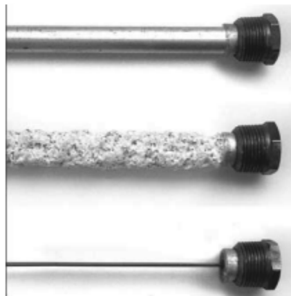
Figure 34 - Anode Rods from new (top) to partially depleted (middle) to fully depleted staged (bottom)
